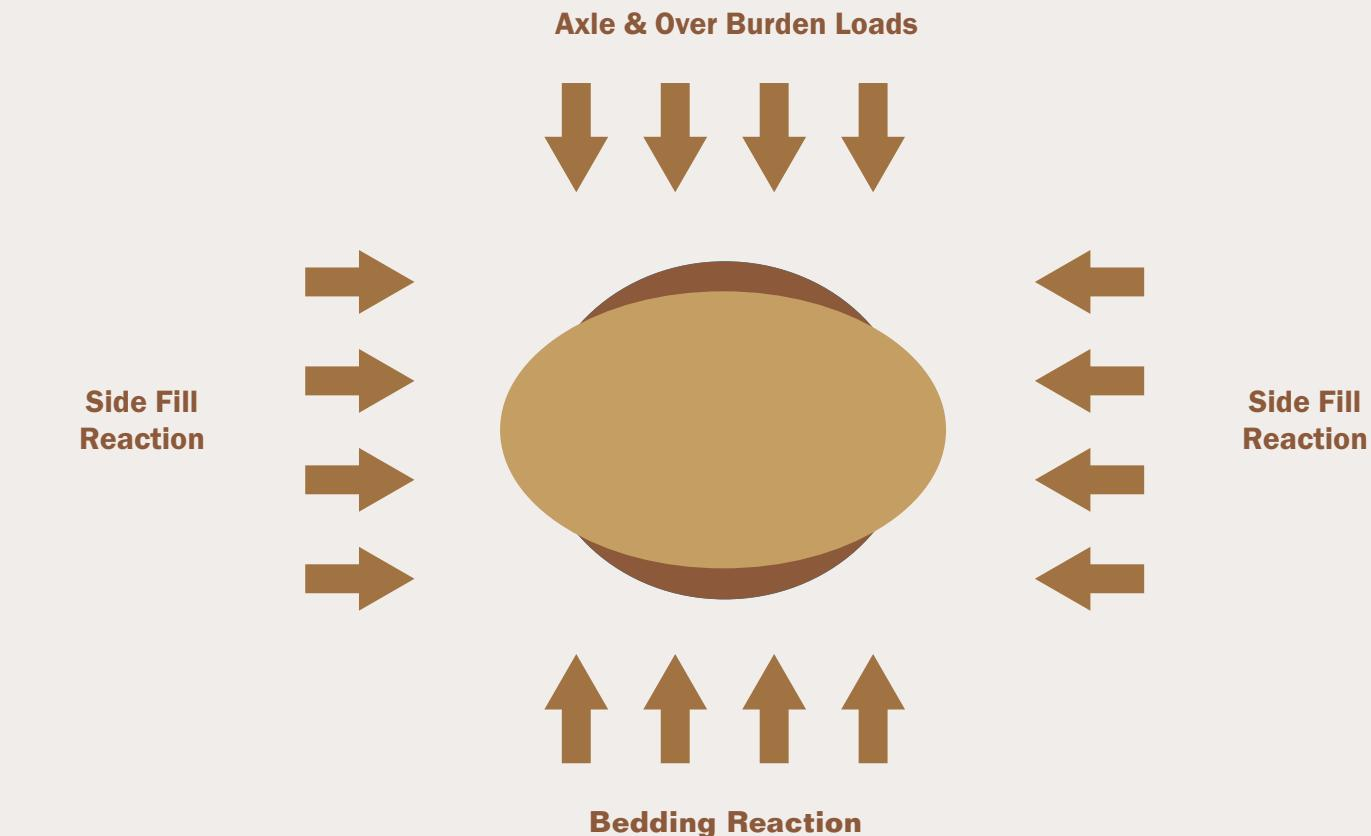
The lateral expansion, as shown above, mobilizes passive resistance in the soil which, in combination with the pipe's inherent stiffness, resists further lateral expansion and consequently further vertical deflection.
